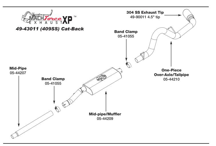
**Step 1:** (Read Instructions prior to installation) Remove your stock exhaust up to the catalytic converter from the rear of your truck working your way forward. Take caution not to damage the factory band clamp and isolation mounts as they will be reused. **It is recommended to not fully tighten the clamps until the entire system has been installed.**
