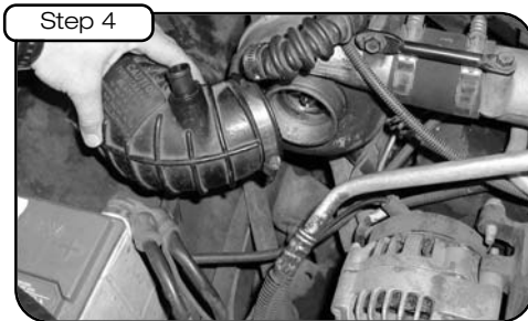
Remove factory rubber elbow at turbo.
