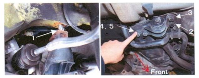
4. Please match the imprinted part numbers on each collar to the appropriate position and orientation shown in the diagram.
