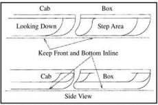
**8A.** Make sure cab and box boards line up. Always mount cab boards first.
