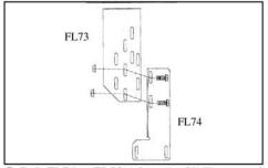
5. Bolt FL74 to FL73 using two 5/16" nuts and bolts in slots shown.
