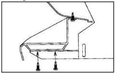
Attach GlaStep to bracket using two #14 x 3/4" self-drilling screws per support. Adjust height of step, then tighten all bolts.
