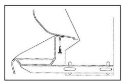
8. Position step on bracket aligning step with cab step. Attach to box using three #12 x 1-1/4" self-drilling screws with rubber washers.
