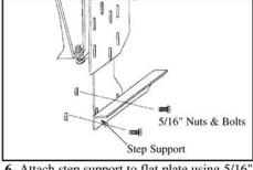
**6.** Attach step support to flat plate using 5/16" nuts and bolts. **Do not tighten at this time.**
