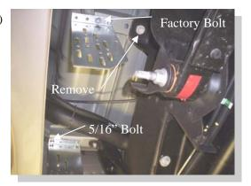
Attach FL73D on bed cross members as shown using 5/16" bolt into inserted clip nut and factory bolt back into fender brace. Use one 3/4" long self drilling screw in each bracket. Remove bed mounting bolt.
