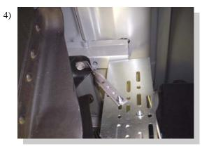
Attach twisted strap using bed mounting bolt removed in step two and one 5/16" bolt and nut as shown.
