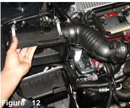
Figure 9 Loosen the clamp on the plastic air inlet tube.
