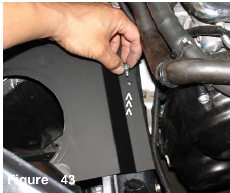
Figure 43 The heat shield bolt hole on the step side is lined up to the pre-tapped hole in the frame. Use the m6 x 12mm bolt in the kit to secure the heat shield.
