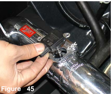
Figure 45 The mass air flow sensor is carefully inserted into the machined sensor flange. Use a dab of light oil around the O-ring to prevent it from kinking or tearing.
