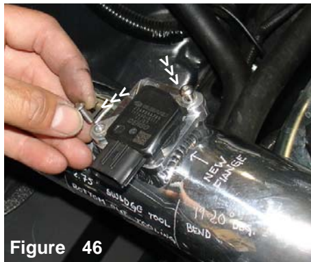
Figure 46 The stock screws are used to fasten the mass air flow sensor to the machined sensor adapter.
