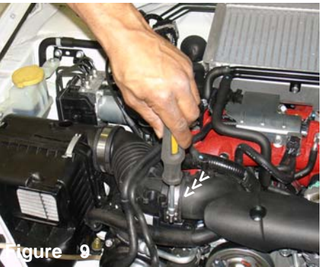
Figure 6 The electrical harness clip is disconnected from the mass air flow sensor.
