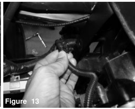
Figure 13 Locate the harness clip connected on frame near head light and remove, this will be used for the vibra mount.
