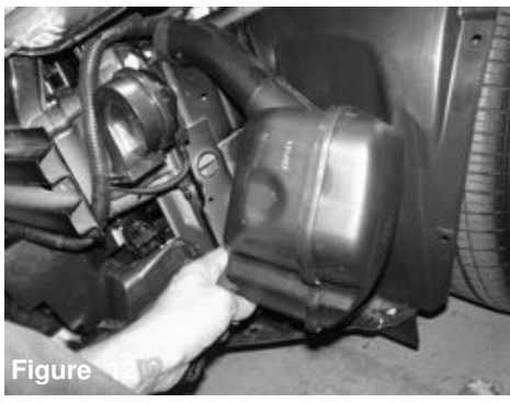
Figure 12 Carefully remove the resonator box out of vehicle.
