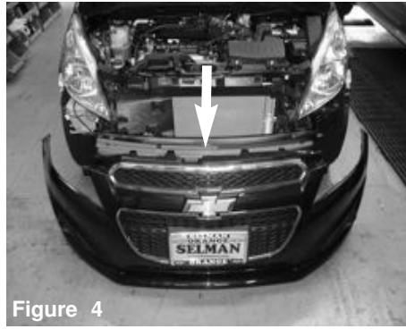
Figure 4 Removal of front bumper cover is necessary. remove top and bottom screws of bumper cover and side screw under head light near fender line.
