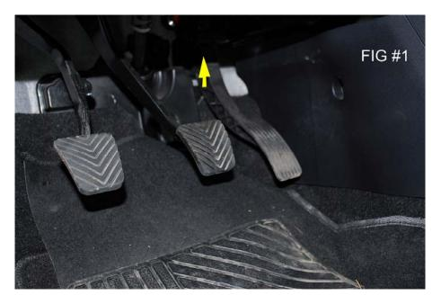
Some Lancer and Evo cars, depending on assembly specs, may have a protective shield just above the pedal. Three plastic pull rivets will release this shield of its location where it meets along the bottom of the dash under the steering column.
