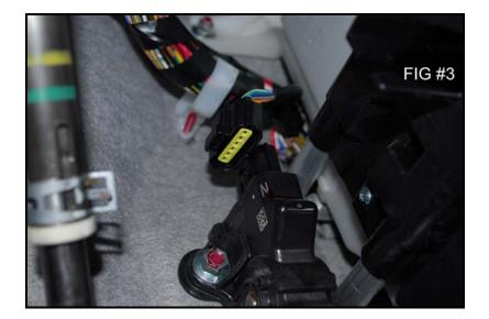
Step 3- Once the harness is free of the pedal, place inline the Sprint Booster. Fig #4 shows the proper installation position with harness reattached. When inserting the Sprint Booster, be careful not to use excessive force or misalign while pressing it in. This can damage the pins of the connector. The Sprint Booster can only be installed in one direction successfully. The tab on the Sprint Booster goes downward and to the driver side of the connection.
