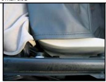
THE FRONT STRAPS HOOK INTO THE BOTTOM OF THE QUARTER TRIM PANEL JUST ABOVE THE SEAT BELT BRACKET
