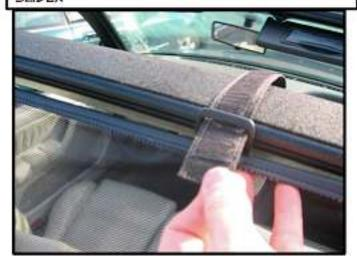
PULL THE STRAP SNUG AND THEN FOLD THE STRAP SO THE VELCRO ON EACH SIDE OF THE STRAP IS HELD IN PLACE
